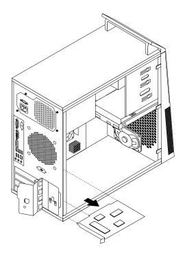
Figure 12. Removing a PCI card
